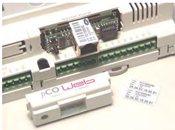
Inserting pCOWeb in the pCO
