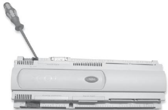
remove the "clock card" placement cover with a screwdriver
